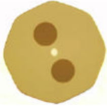
Fig. 4. Cross-section of a 20micron core, 400micron inner-clad Panda-type ytterbium-doped PM-LMA-DCF.
